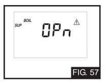
The control is no longer able to read the boiler supply sensor due to an open circuit (FIG. 57). The control will not operate the boiler(s) until the sensor is repaired. Locate and repair the problem as described in INS7141. To clear the error message from the control after the sensor has been repaired, press either the Menu or Item button.
